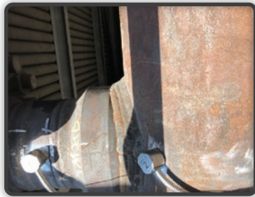
Dual-Element UT sensors with optional SS cable jacket
