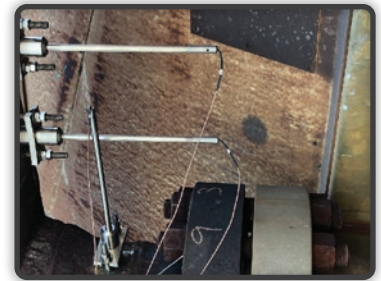
Ultra-High-Temp UT Sensors attached with stud welded clamp
