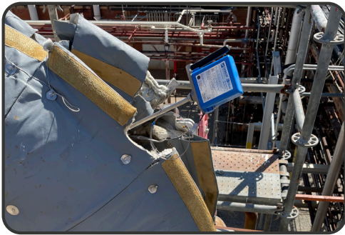
microTEMP attached with a band clamp out of insulation
