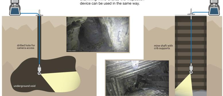
SNI offers three different camera heads for the HI-DEF PTZx. The 3" camera will easily navigate a hole three inches or greater.
