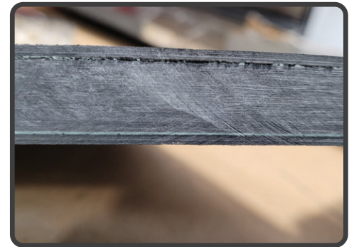
Cross-Section of defect from an Ultrasonic Indication
