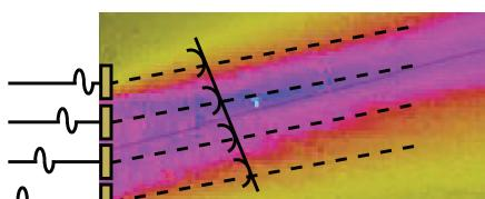
By alternating the timing sequence of the pulses, the direction of the transmitted beam can be varied to any desired scan angle. This allows for multiple angle inspections, using a single transducer. The **maximum steering angle** (at -6 dB) in a given case is derived from the equation:
