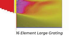
The beam is electronically focused by applying symmetrical delay laws to the different elements of a transducer. This technique can be combined with beam steering to produce both angled and focused beams.
