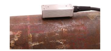
**Corrosion Mapping:** Dual-linear arrays in 16 or 32 pairs of send / receive elements combined with replaceable delay lines are perfect for scanning large surface areas for pitting or general corrosion / erosion.
