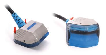
Rotor Disc: High-element count linear array with couplant irrigation ports and compound-radii integral wedge for scanning of aerospace discs.
