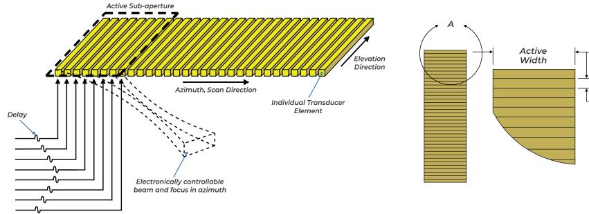
This shows a linear array geometry showing electronic control over a sub-aperture of the array which allows electronic control of the beam. Elevation performance is fixed by the frequency, aperture size, and the potential addition of a focusing lens.
