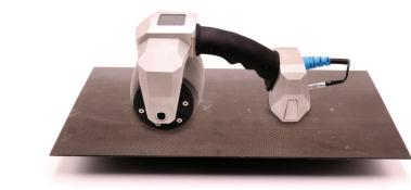
**Composite Material:** 32-or 64-element linear array configured in a captive water column, the compliant WheelArray is used with minimal couplant for inspecting aerospace and wind blade composite components.
