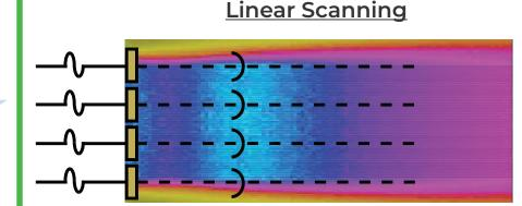
The beam is electronically translated by alternately firing a given number of elements of a phased array transducer. Only one angle is introduced but is introduced multiple times throughout the length on the array.
