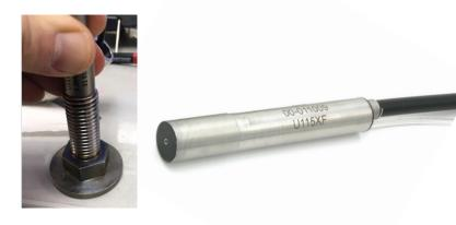
**Bolts:** Round, segmented-annular arrays are ideal for the interrogation of threaded zones on studs and bolts of almost any size.
