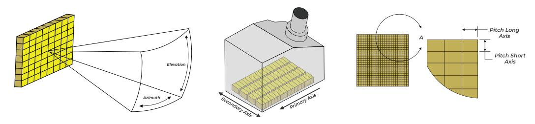
Active aperture =  $(N \times P Primary axis) \times (N \times P Secondary axis)$ N = number of elements in the transducer *P* = element pitch
