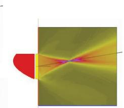
The **active aperture** is one of the critical features used to define a phased-array transducer. It is the total active transducer length, and can be calculated by the following formula:
