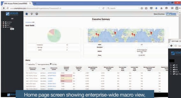
Home page screen showing enterprise-wide macro view, including pie chart with sensor location, status, GPS and latest readings of all sensors.
