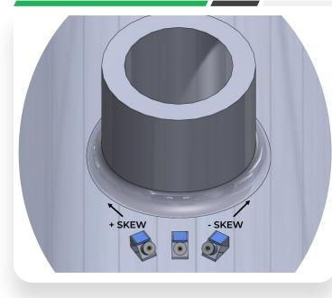
The Wedge - UT wedges are used in industrial NDT inspections to introduce the transducer's acoustic energy at a non-perpendicular angle thereby allowing the sound beam to be transmitted at a more-optimized angle within the test part. The wave mode and angle is selected to maximize the ability to identify and size defects based on the test part's material, defect type, and orientation.
