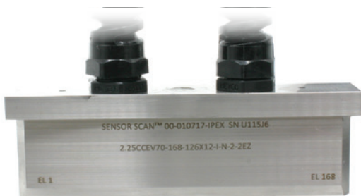
2.25MHz | 168 element Linear Array 0.75mm Pitch | 12mm Elevation
