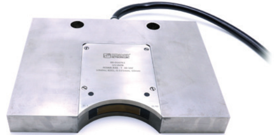
10MHz | 82 element | Curved Linear 0.515mm Pitch | 10mm Elevation
