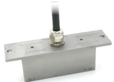
3.5MHz | 64 element | Linear Array 1mm Pitch | 7mm Elevation
