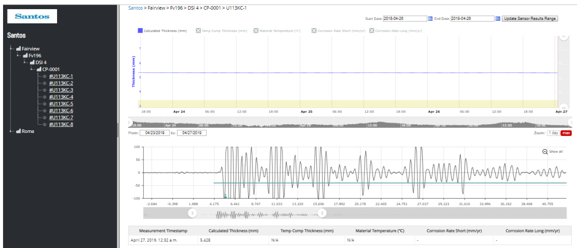
The metal loss plot, shown above, was 0.001" for a seven-day period which, if left unabated, would be 0.060" year. Installed sensor systems can accurately identify trends more rapidly therefore enabling faster intervention.
