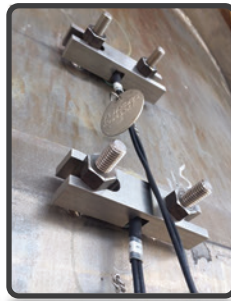
Non-magnetic vessel monitoring with "duals" via stud-welded brackets.
