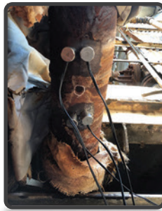
XD-101 and XD-301 attached with magnets
