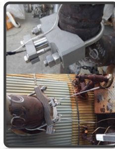
XD-201 probes attached with U-bolt
