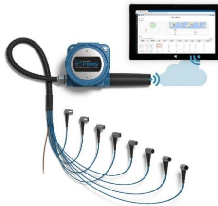
Battery powered, self-contained 8 dual-element cellular system can be programmed to take UT thickness measurements at any user-defined time interval. Data is sent to a web portal where it is trended.
