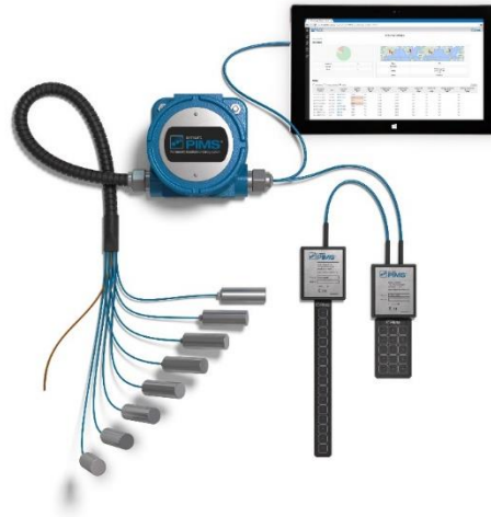
Illustration of a wired, multi-drop Modbus system for UT thickness data collection over a large area.
