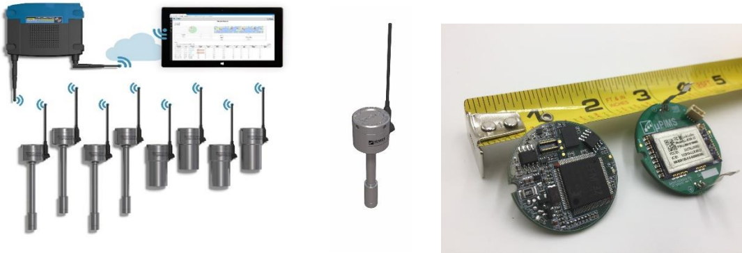
Example of a wireless UT sensor network along with a typical UT thickness & temperature node. The entire UT / wireless system resides on a small printed circuit board (PCB).
