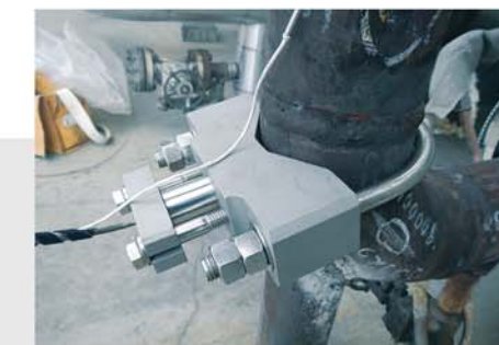
Transducer model XD-201 is an ultra-high temp probe which can operate in 900° F (500°C) continuous-duty service. These probes and their temperature-measuring RTDs are mechanically clamped onto the plant asset.
