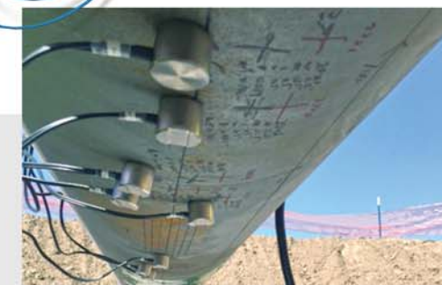
SNI's Pit-track™ hardware/software solution can monitor the growth of many individual pits with a high degree of thickness resolution.
