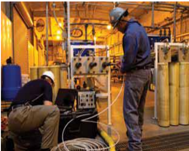
Figure 12 (left): Field inspection of specialized heat exchanger tubes at a chemical plant using eddy current technology.
