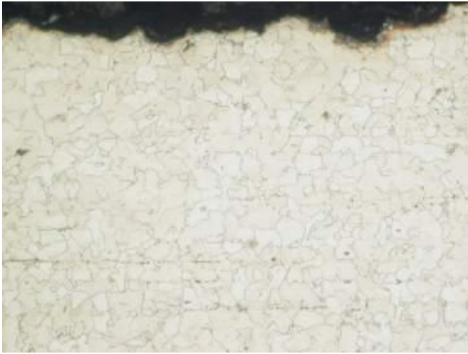
Figure 15 (left): A pipe ID surface exhibiting complete decarburization of the original structure, magnified at 200X.
