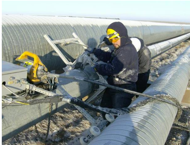
Figure 2: Field deployment of digital x-ray (DXR) imaging system for insulated pipe inspection.
