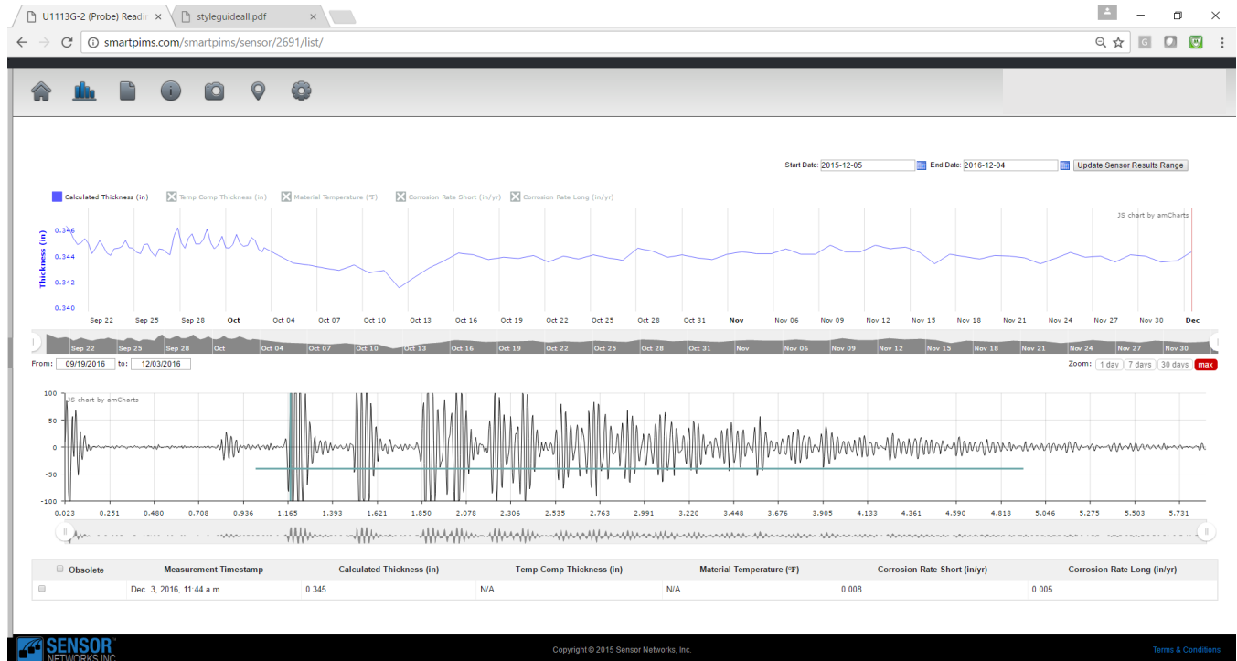
Figure 9: Results of installed ultrasonic monitoring of an overhead crude line.
